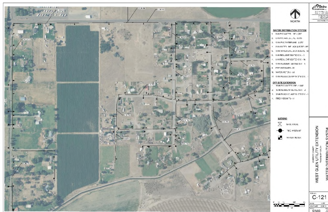
Figure 1: Preliminary Water Distribution System Layout
