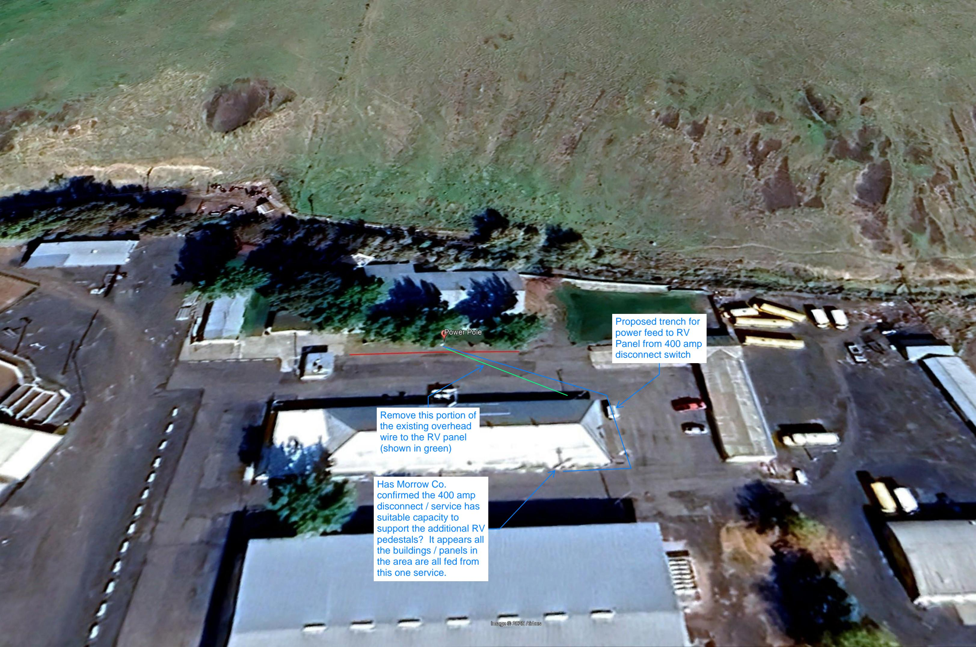
Proposed trench for power feed to RV Panel from 400 amp disconnect switch
