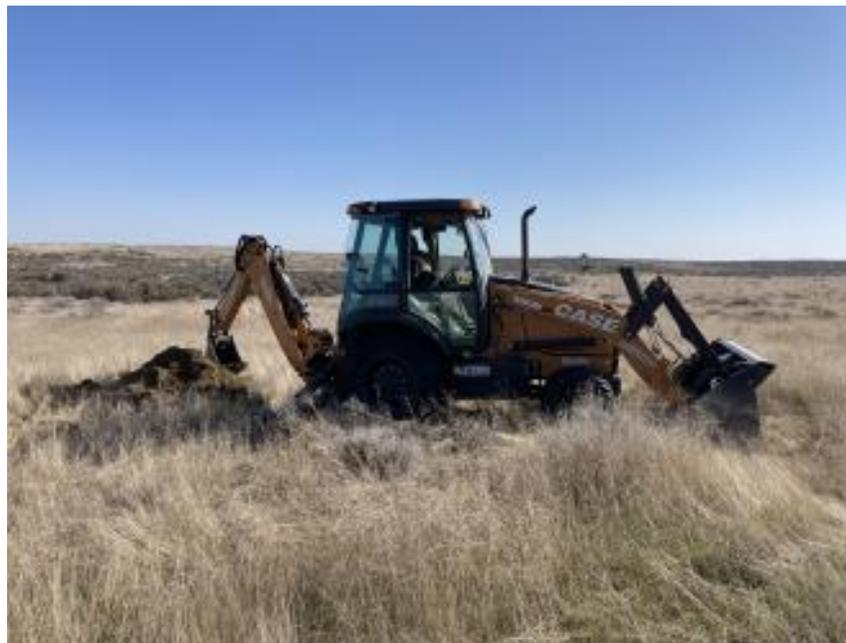
**Photo 4** - Excavator used for digging test pits
