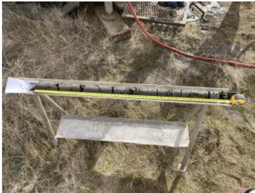
**Photo 3** - Sample from borehole
