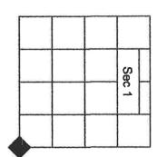
**Description of corner evidence found:**Found the intersection of long standing north, south and west fence. Due to it near record relationship to the surrounding accepted corner positions, accepted this position as best available evidence.
