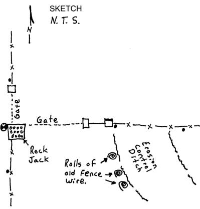
MONUMENT (S) AND ACCESSORIES SET (Procedures and Description) At the fence corner as identified above I set a 1" x 24" iron rebar flush with the surface of the
