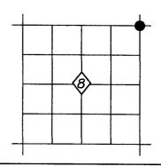
ORIGINAL G.L.O. DESCRIPTION: Set Stone 23x7x6 for corner to Sections 4, 5, 8, 9 on top of flat hill.
