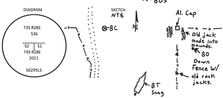
At the position of the original stone I set a 1"x24" iron rebar with a 2" aluminum cap stamped as shown in the diagram above. I buried the original stone upside down on the NE side of the rebar along with the location poster.
