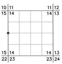
ORIGINAL DESCRIPTION: Set a basalt stone 12x10x7 ins. 8 ins. in the ground, for 1/4 sec. cor. marked 1/4 on W. face from which
