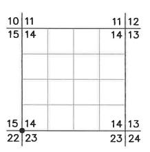
**1884 G.L.O. DESCRIPTION:** Set a post 4 ft. long, 4 ins square, 24 ins in the ground for cor. to secs 14, 15, 22 & 23 marked T4S S14 on N.E., R28E S23 on S.E., S22 on S.W. and S15 on N.W. faces with 3 notches on S. and 2 notches on E. edges, from which
