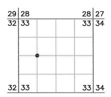
ORIGINAL DESCRIPTION: At the corner point I set a  $2\frac{1}{2}$ "x30" alum. pipe with a  $2\frac{1}{2}$ " alum. cap containing a magnet and marked: (diagram shown) Monument is 25" in the ground.
