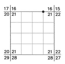
ORIGINAL DESCRIPTION: At the location of this corner, as established by survey, set a 2 1/2 inch alum. pipe, 30 inches long, 2 feet in the ground, with an alum. cap marked as shown above. From this monument as set, A Bearing Tree, a 6" L.P. pine, bears N 33° E, a distance of 19.2 feet, which I marked E 1/16 S16 BT. A Bearing Tree, a 14" Spruce, bears S 8° W, a distance of 48.2 feet, which I marked E 1/16 S21 BT.
