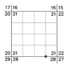
**ORIGINAL DESCRIPTION:** At the location of this corner, as established by a survey conducted by me, I set a 2 1/2 inch alum. pipe, 30 inches long, 2 feet in the ground, with an alum. cap marked as shown above.
