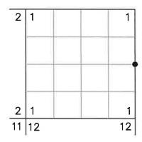
ORIGINAL DESCRIPTION: A fir 6 in dia for 1/4 sec cor. from which a pine 8 in dia. S.30°E. 21 lks.
