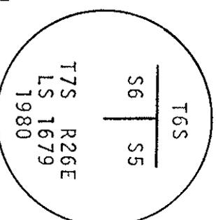
I deposit the original stone alongside as a memorial and take the following trees and take the measurement to the center of the tree at the lower blaze in which I place a brass washer stamped LS 1679:
