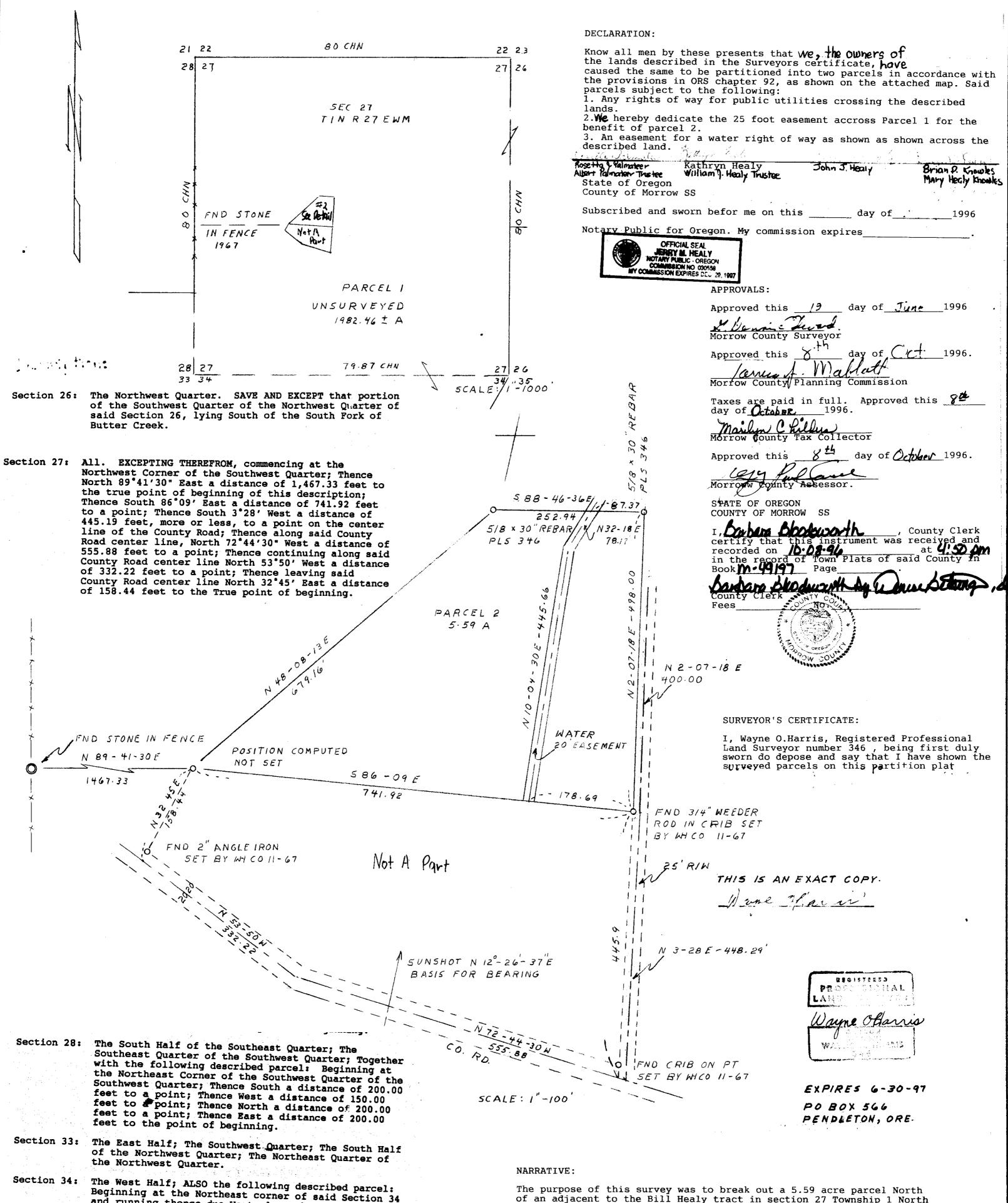
The purpose of this survey was to break out a 5.59 acre parcel North of an adjacent to the Bill Healy tract in section 27 Township 1 North , Range 27 East of the Willamette Meridian. I found points from a survey made by this company in November of 1967. I made a sunshot as shown and used these points to control the survey shown above
