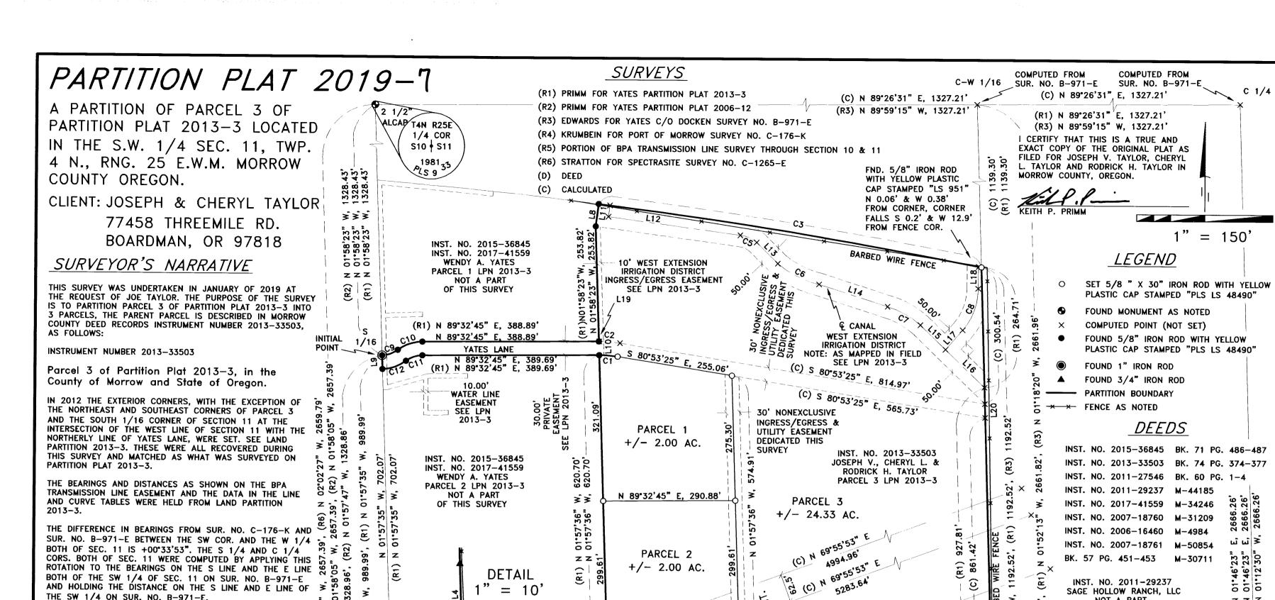
THE W 1/16 AND THE C-W 1/16 CORS. BOTH OF SEC. 11 WERE COMPUTED AT THE MID POINT OF THE S LINE AND AT THE MID POINT OF THE N LINE BOTH OF THE SW 1/4 OF
