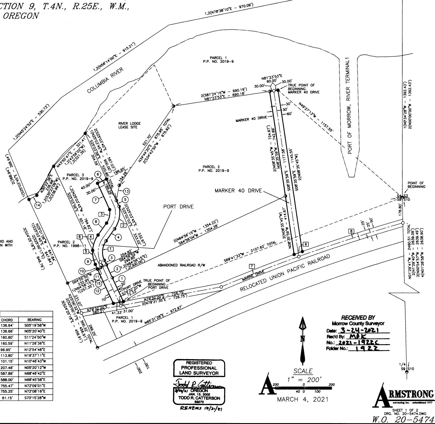
ROAD DEDICATION SURVEY OF PORT DRIVE AND MARKER 40 DRIVE ACROSS PARCELS 1 AND 3 OF PARTITION PLAT NO. 2019-9 AND PARCEL 2 OF PARTITION PLAT NO. 1998-11 LOCATED IN THE SE1/4 OF SECTION 4 AND THE NE1/4 OF SECTION 9, T.4N., R.25E., W.M., CITY OF BOARDMAN, MORROW COUNTY, OREGON W.O. 20-5474
